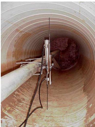
**FIGURE 2** Measurement system installed inside a pipe.
