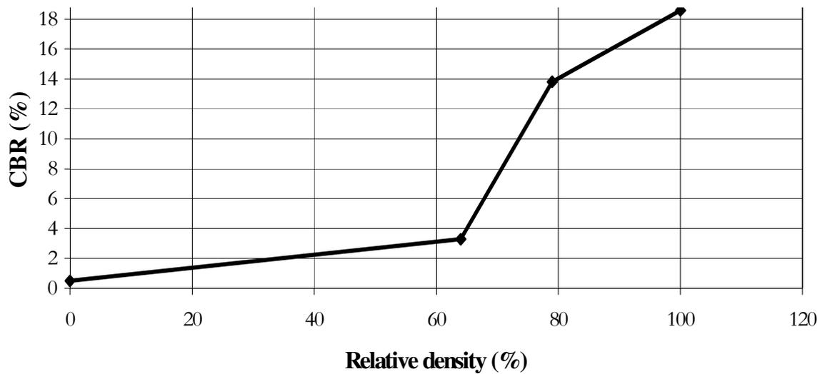
**FIGURE 5 CBR in function of relative density for the tested sand.**
