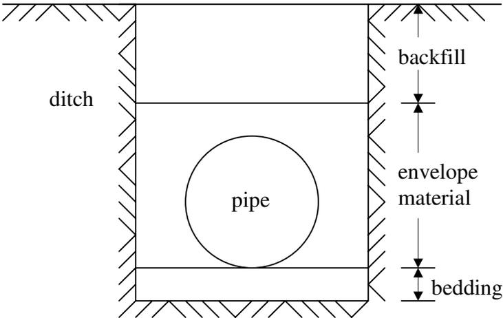
**FIGURE 1 Schematic representation of a buried pipe.**
