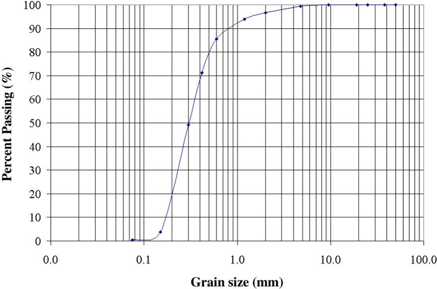
**FIGURE 4 Grain-size distribution of the tested sand.**
