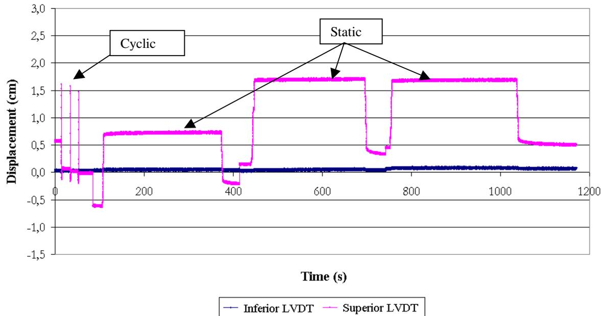
**FIGURE 6** Pipe vertical displacements under 60kN wheel load for the compacted shallow ditch.
