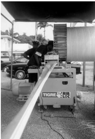
**FIGURE 3 Ribbed flexible plastic pipe being spirally wound.**
